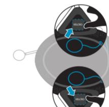
Attach the Velcro Pads to the helmet's inner padding
