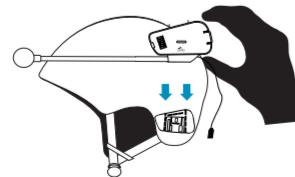
Slide the back plate into position on the glue plate
